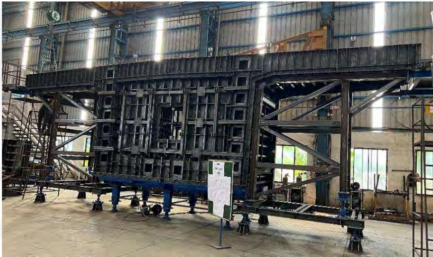
Pier Head Segment
